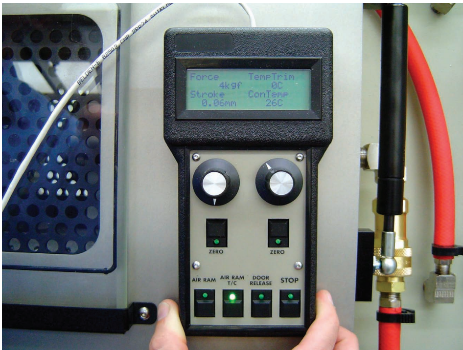
The Gleeble Pendant is extremely useful whenever you need to operate away from the Gleeble console.
