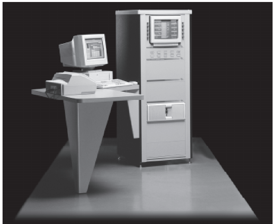
The Gleeble 1500 Digital Control System is shown above with optional computer table.
