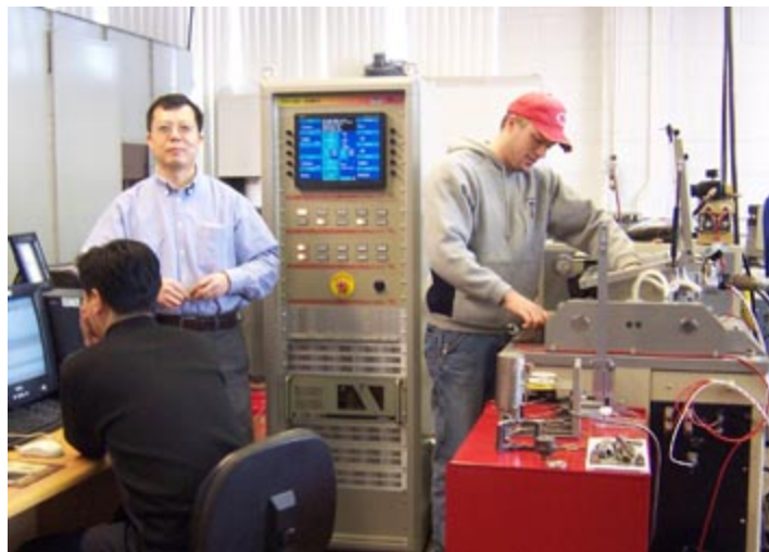
Dr. Leijun Li and colleagues at Utah State University use a Gleeble physical simulation system to perform severe deformation on powdered lithium amide to fabricate nano-scale hydrogen storage materials.
