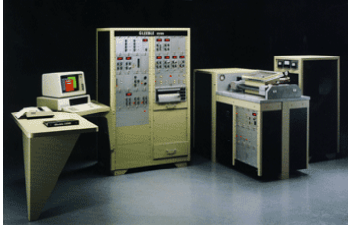
The Gleeble 1500, manufactured from 1979 to 1995, was the first system to feature PC-based controls and closed-loop servo hydraulics with high-speed direct resistance heating. This combination provided a platform for new physical simulation applications.
