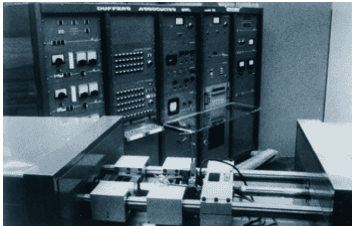
The Gleeble 512, manufactured during the 1970s, was physically the largest Gleeble built until the Gleeble 2000 was introduced in 1990. This model featured direct resistance heating and had an open loop mechanical system for high-speed tensile tests.
