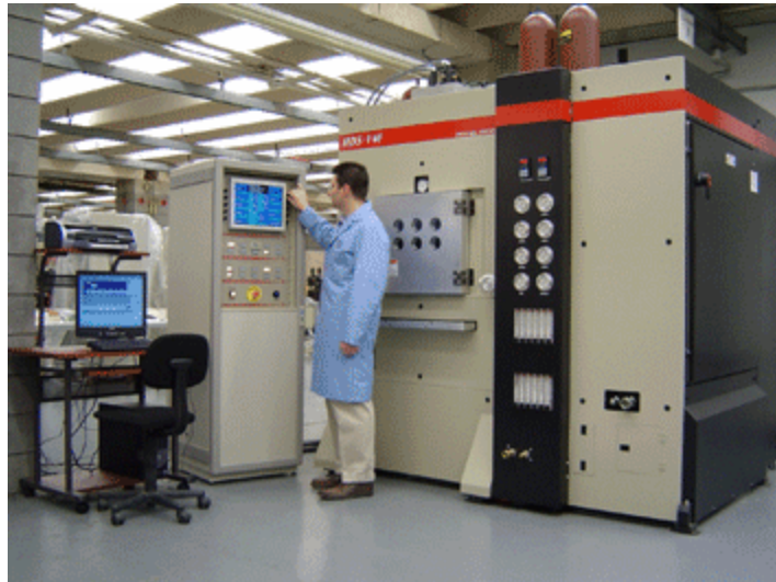
The HDS-V40, introduced in 2004, is capable of simulating direct rolling, from the continuous caster to the end of the hot rolling process, all in one continuous sequence.
